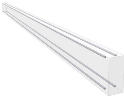
Figure 1.2 reinforcement in KLP®-S beams
