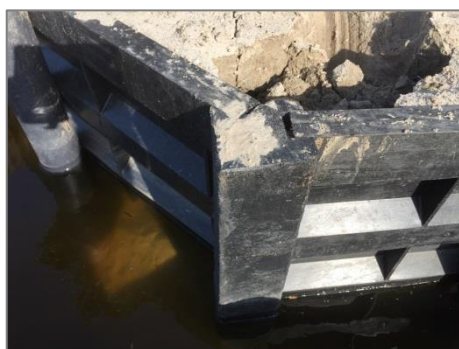
KLP® Pole for RapidRetain corner solution. Supplied with recess on 1 side (50x40mm). The contractor has to mill the other recess in the right angle on location.
