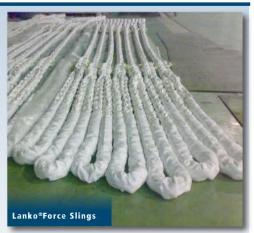
At present Lankhorst offers the Lanko®Force 12 x 1 construction and standard 12 strand ropes to produce slings with a minimum breaking load (MBL) of around 1,600 mT in single leg configuration and 2,700 mT on a grommet configuration.
